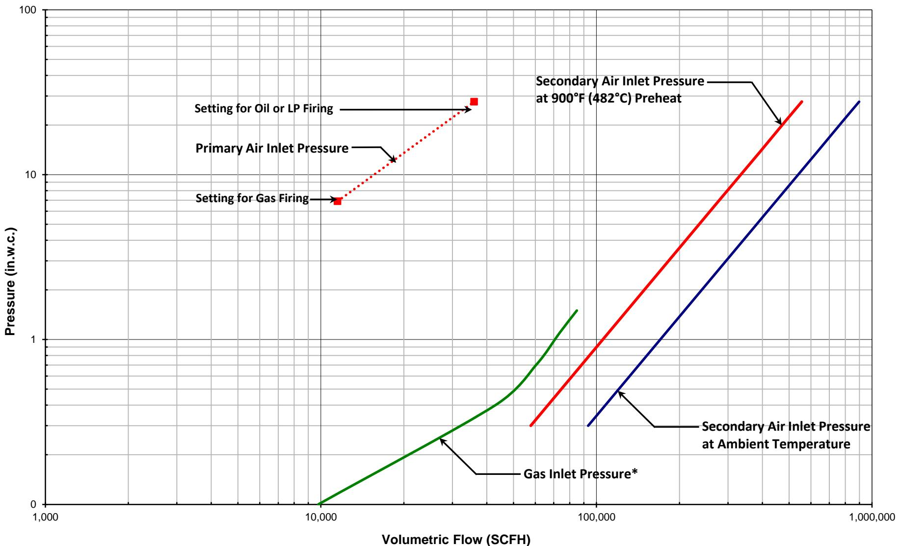
\*Note: Gas Inlet Pressure for HBC burner is not suitable for fuel flow measurement and is given for component sizing and reference only
