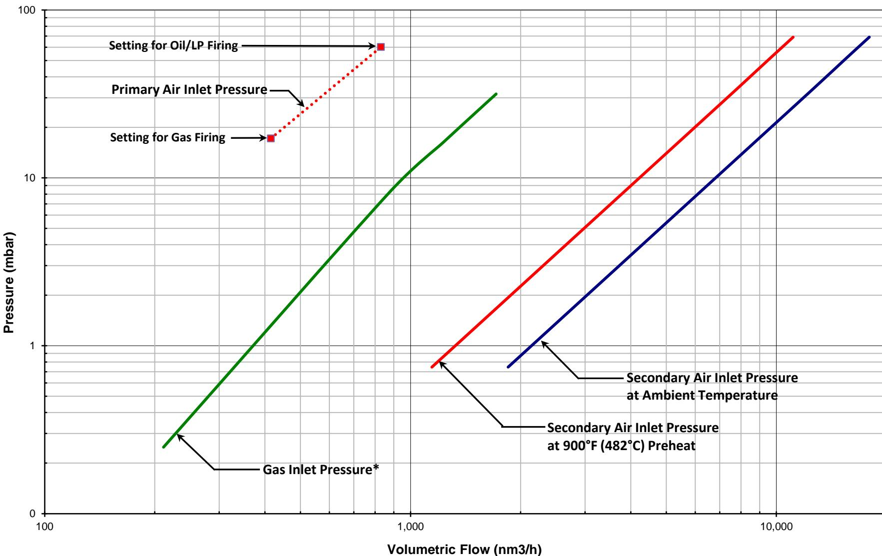
\*Note: Gas Inlet Pressure for HBC burner is not suitable for fuel flow measurement and is given for component sizing and reference only
